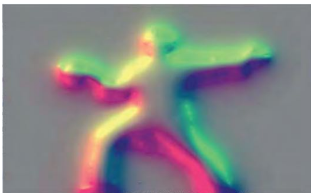
Figure 5 - Force topology map of the human form. Gray indicates a gradient of zero. The intensity of each color is related to the magnitude of the local force vector on the depth image. Color choice has been selected to effectively illustrate depth
